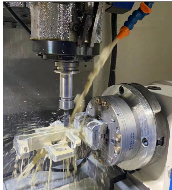
• 四轴搭配R系卡盘强力夹持重切削应用 Heavy-Duty Cutting 4-Axis Machines Equipped with R-Series High-Power Chucks
