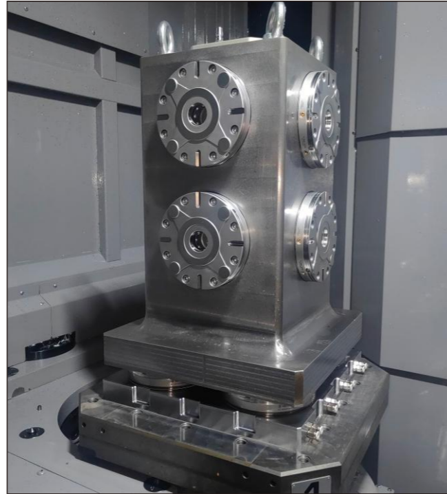
• 卧加方箱零点组合应用 Application of a Modular Fixture System with Zero-Point Clamping on a Horizontal Machining Center
