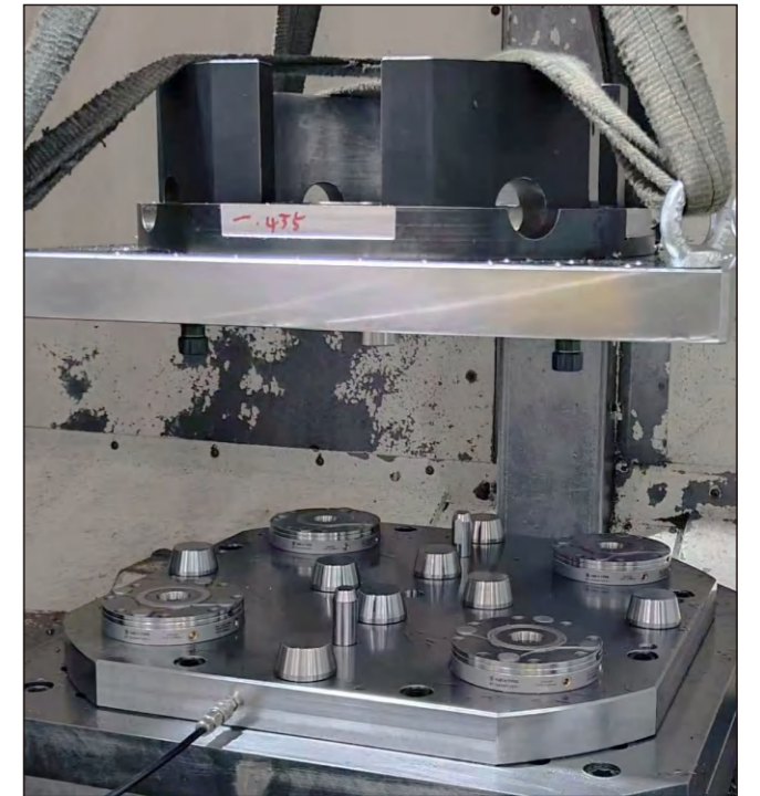
• 大型零件卧式加工中心零点应用 Application of a Heavy-Duty Zero-Point Clamping System on a Large-Part Horizontal Machining Center
