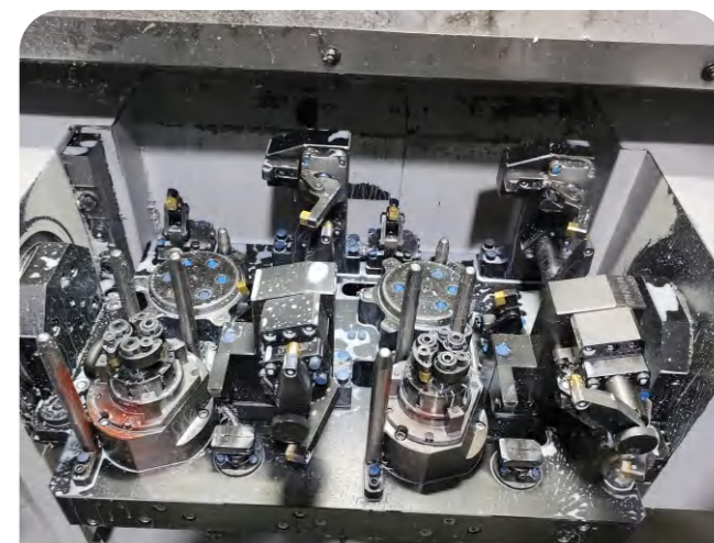
壳体主轴转台液压夹具 Hydraulic Rotary Fixture for Housings/Spindles
