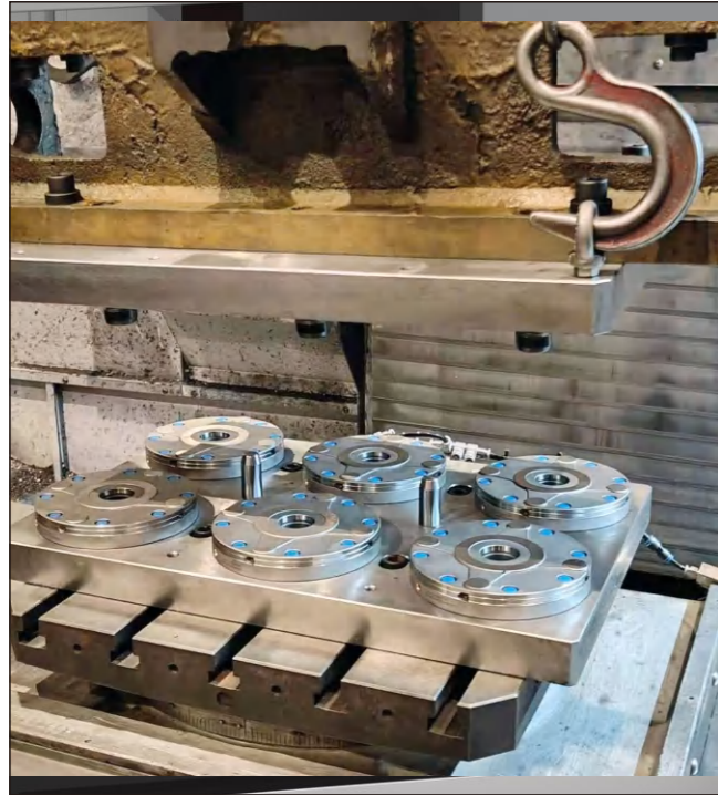
• 六位零点组合大型零件卧式加工中心应用 Application of a Horizontal Machining Center with a Six-Position Zero-Point Clamping System for Large-Part Manufacturing
