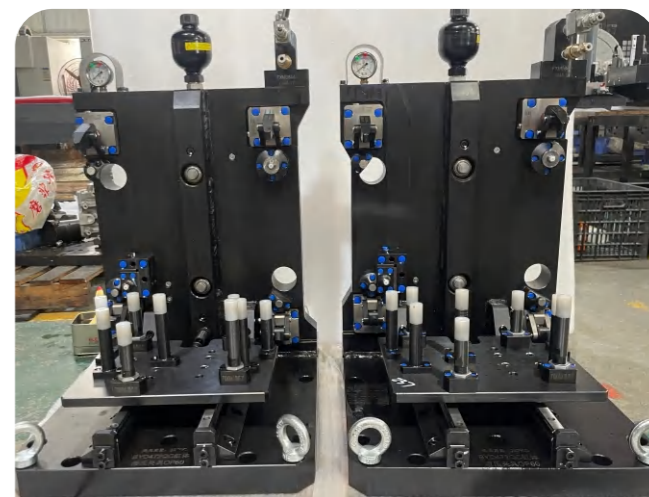
新能源汽车增程发动机缸体液压夹具 Hydraulic Fixture for Range-Extender Engine Block (New Energy Vehicles)
