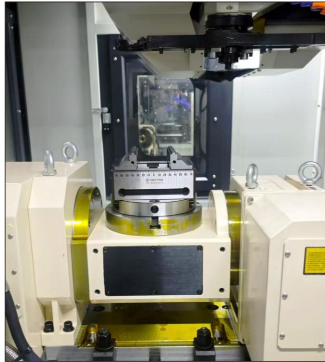
• 手动快换板+定心钳五轴机应用 Manual Zero Point Plates with Self-Centering Vises on 5-Axis Machining Centers
