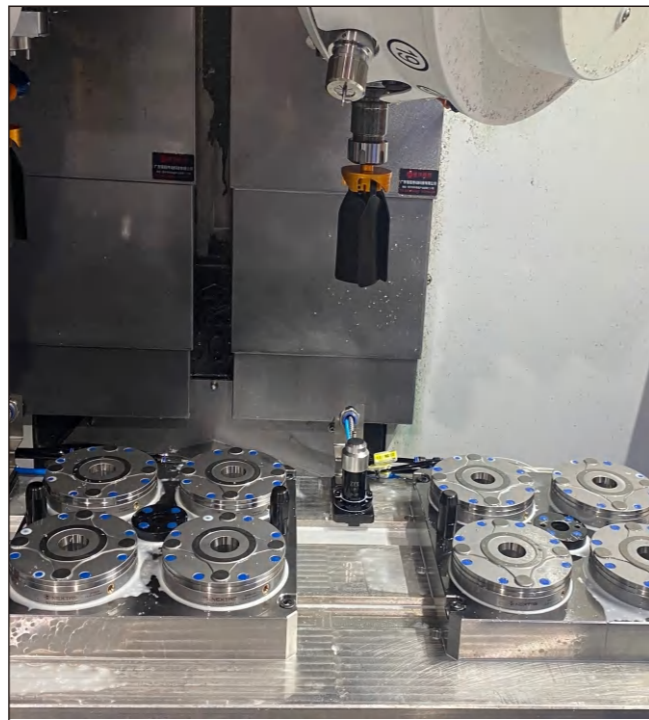
• 三轴立加零点应用 Application of a Zero-Point Clamping System on a 3-Axis Vertical Machining Center (VMC)
