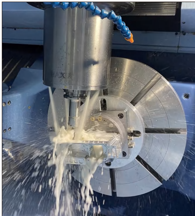
• 五轴搭配R系强力夹持重切削应用 Heavy-Duty Machining 5-Axis Centers Coupled with R-Series High-Power Chucks
