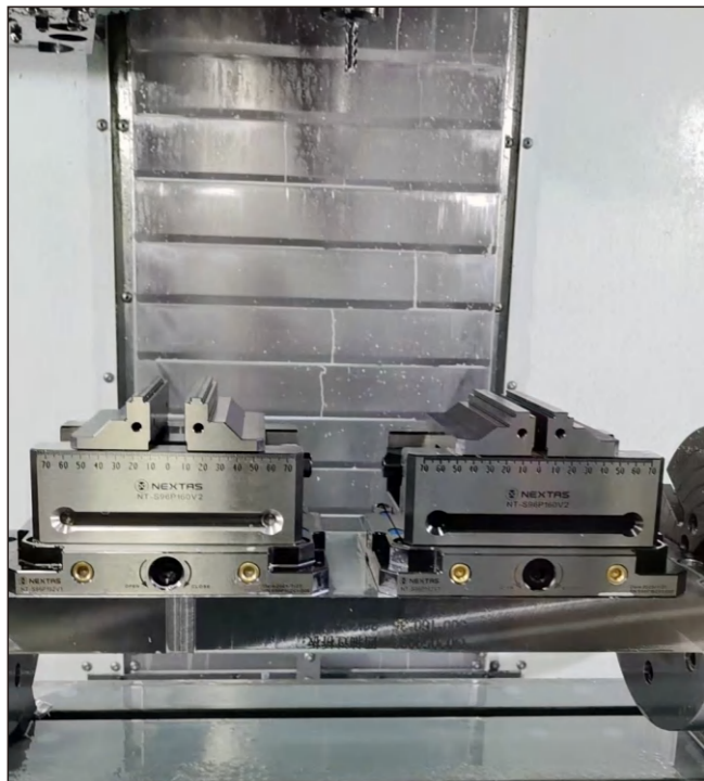
• 手动快换板+定心钳四轴机应用 Manual Zero Point Plates with Self-Centering Vises on 4-Axis Machining Centers
